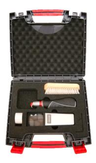
The CHC-520 Cross Hatch Cutter tests the adhesion of a dry coating onto the substrate to which it is applied.
