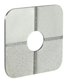
A precision Nickel Comparator Plate that conforms to International Standard ISO 8503 and ASTM D4417 for grit and shot blasted surface roughness comparison.
