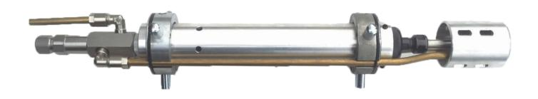
PIPECOATER-III tools are designed to coat the inside of pipe or tubing without the need to rotate pipe or tubing and to apply an even paint film thickness throughout. Generally, any type of coating may be used in this tool that can be airless sprayed. To obtain the best possible production, one man should operate the Control Gun while another man pulls the tool through the pipe or tubing.
