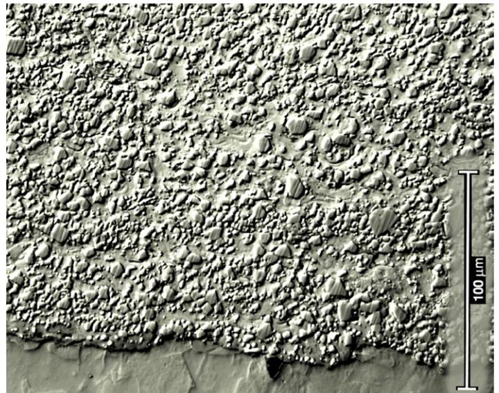
Figure 11 – HVOF spray coating of WC 12(CoCr)
