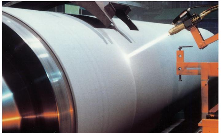
Figure 22 – HVOF coating of a sink roll
