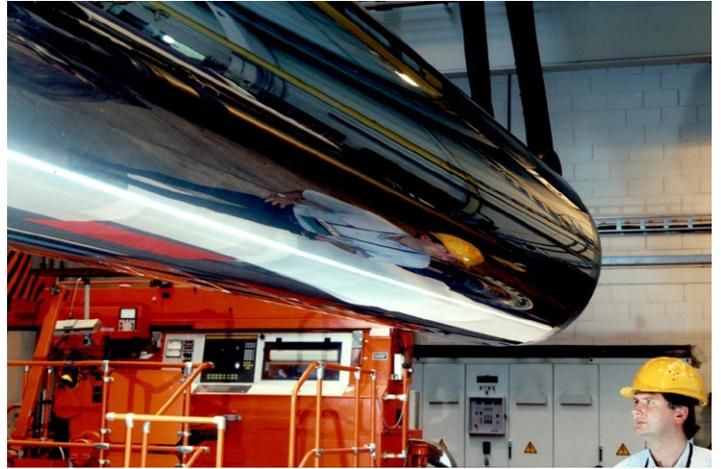
Figure 23 – Metco™CAL coating after superfinishing
